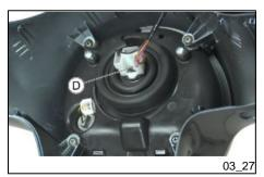
This gives access to the bulbs. Turn the clip and take out the bulb of the high-beam/ low-beam headlamp «**D**».
