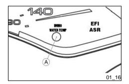
Activation of the "PIAGGIO IMMOBILIZER" system is signalled by a flashing «A» indicator. In order to reduce battery discharge, the indicator LED turns off automatically after 48 hours of uninterrupted functioning. Should the system fail, different LED flashing patterns will provide the **Authorised Service Centre** with information on the type of fault detected.
