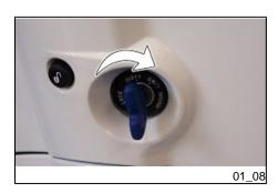
Releasing the steering wheel (01\_08)
