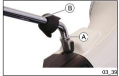
To remove the rear view mirror, lift the rubber protection, unscrew the lock nut **«A»** slightly to unlock the stem. Unscrew the stem **«B»** until removing it.
