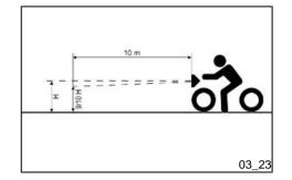
**2**. Turn on the headlight and check that the borderline of the projected light beam on the screen is not lower than 9/10 of the distance from the ground to the centre of vehicle headlamp and higher than 7/10;
