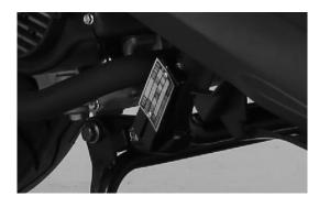
The product nameplate is riveted on the right lower part of the frame.
