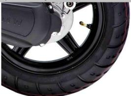
Check the pressure of the rear tire. Set between 35 and 40 Psi. Check for abnormal wear on the tire tread and outer walls.
