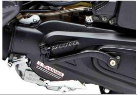
3)Pull out the foot lever, place your foot on it and push firmly and quickly all the way down. Let the arm return to its horizontal position before you try to kick start it again. Repeat this motion.
