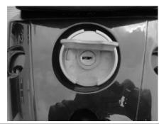
Ensure you have enough gas for your trip and ensure the gas cap is secured properly.
