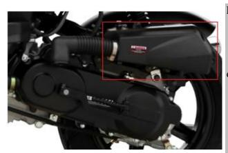
Remove the screws for the air filter cover, and remove the cover. Check whether there is dust and dirt on the foam of the filter element. Remove the air filter and wipe off the dust inside the air filter with clean and dry cloth.
