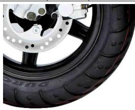
Check the air pressure of the tire and visually inspect the rubber tire and rim for excessive wear or defects. If there are any issues, the tire should be replaced at a local authorized service center.
