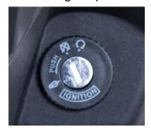
Turn the ignition on and ensure all turn signals and other lights are working.
