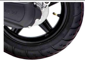
Check the tread wear depth of the tire and inspect for damage. If any abnormality is found, the tire must be replaced immediately.
