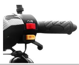
While holding either brake handle, push the electric start button with your right thumb. Use the accelerator a small amount with your right hand to add an appropriate amount of fuel.
