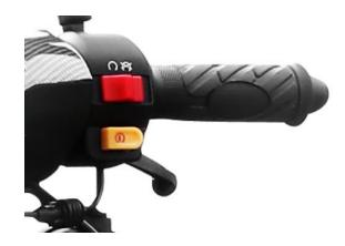
Check that the throttle grip rotates smoothly and freely. If not, the throttle cable may need lubrication or replacing.
