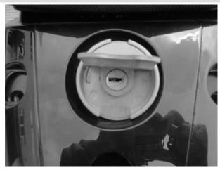
Closing the fuel cap: Insert the fuel cap in the fuel tank opening and turn it clockwise. Once it is closed fully, you can remove the key and flip the tab down.
