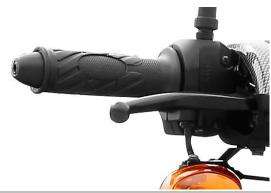
Front brake: This is the right lever when you're sitting on the vehicle. It uses a disc brake.
