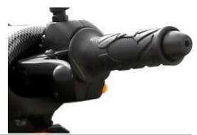
Rear brake: This is the left lever when you're sitting on the vehicle. It is a drum brake.
