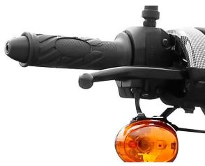
\* Check the travel of the brake lever when applied. Excessive travel could indicate worn pads or air in the brake fluid. Either of which need to be addressed prior to riding.
