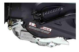
The Engine Number is printed on the left lower part of the crankcase.
