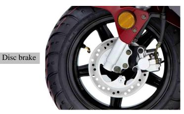
\* Check for the wear on the front disc rotor. Any signs of warping or irregularities in the surface of the brake rotor can cause vibration, lower braking force, and increase the stopping distance. Replace if needed.
