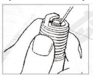
Correct spark plug gap helps fuel economy and performance. Incorrectly gapped spark plugs can lead to hard starting and poor performance. Always replace the spark plug with the original NGK replacement. These are pre-gapped from the factory
