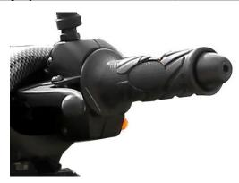
Check that the rear brake lever has the correct amount of free play in it. About 20-30 mm. (0.787-1.181 inch)
