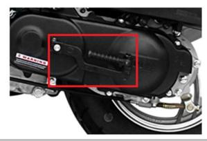
Kick Starter: This is used for manually starting the engine. The vehicle must be on the main stand, the ignition must be on and the brake levers need to be held in while you kick start the engine.
