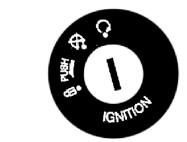
First, insert the key into the ignition switch lock, and turn it to the "position."
