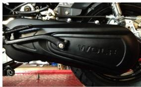
Automatic clutch: The CVT allows smooth acceleration without the need for gear changes.
