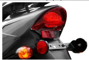
Check that the tail light and brake lights work properly.
