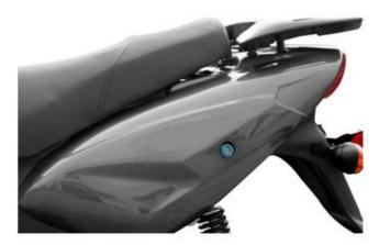
Seat: Insert the ignition lock key into the seat lock and turn it clockwise to open the seat.
