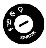
To lock the steering column, turn the handlebars all the way to the left, push the key inwards and turn the ignition to the "position to prevent the vehicle from being stolen easily.
