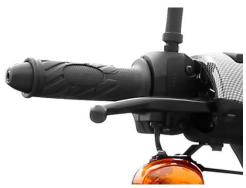
2)The vehicle should be put on the main stand and you need to hold the brake levers to allow the engine to start.
