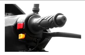
4)Twist the throttle slightly to allow more gas flow as you kick the engine over. Once started, let the engine warm up before revving the engine at high RPM.
