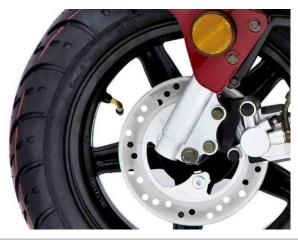
Check the pressure of the front tire. Set to between 35 and 40 Psi. Check for abnormal wear on the tire tread and outer walls.
